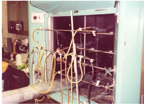
FIGURE 2. Smoke Test Using SKC Smoke Tubes
