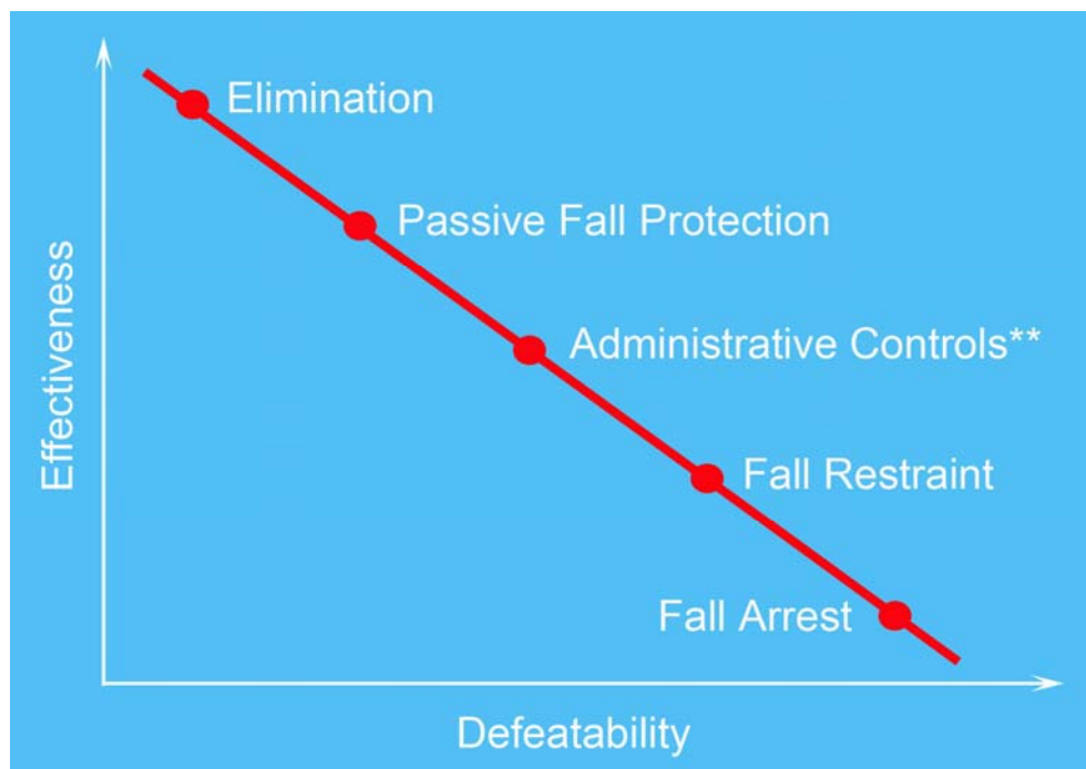
Exhibit 2. The Hierarchy of Controls relates hazard abatement options in terms of effectiveness and ability to be defeated.
