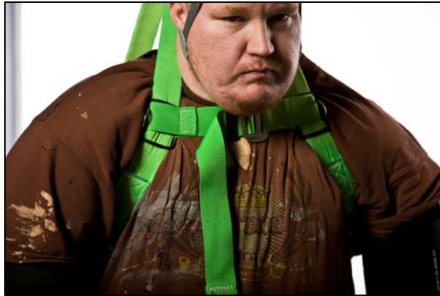
Exhibit 3. Several of the harnesses encroached on the neck.
