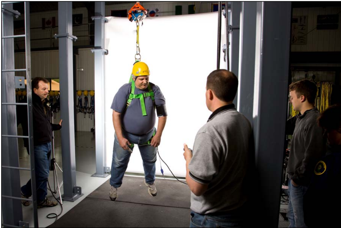
Exhibit 1. Volunteers were fitted with full-body harnesses and suspended 6” from the ground.
