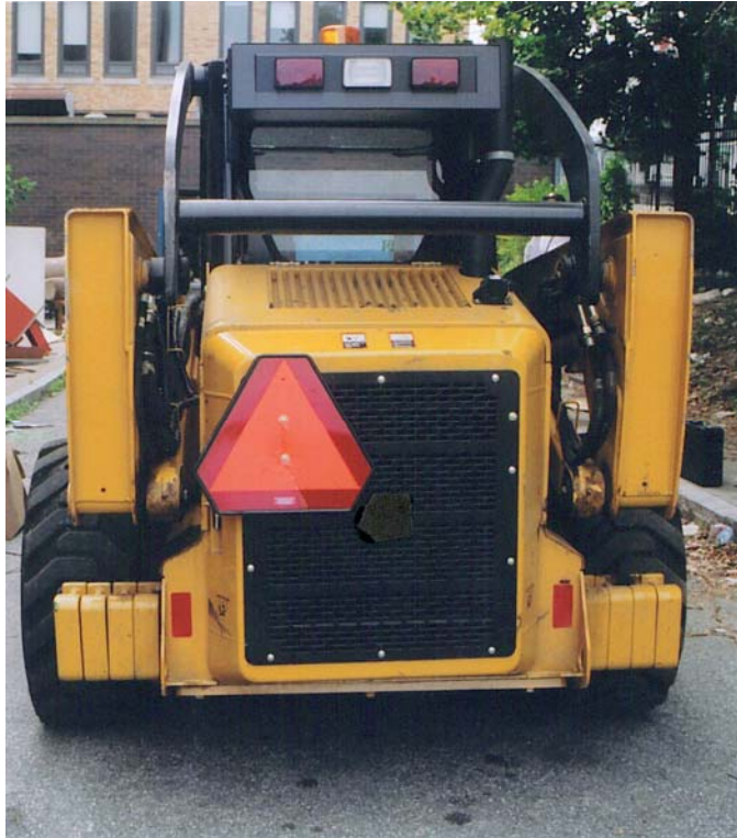
Exhibit 2. This photo shows a loader equipped with a rollover protection structure (ROPS).
