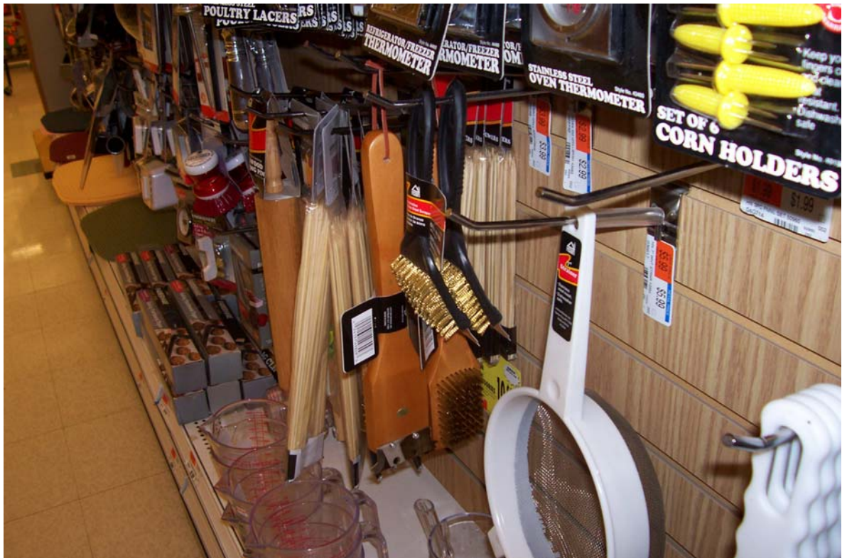
Exhibit 7. This photo shows a typical merchandise display used in many retail stores. The display hooks are dangerous because the pointed end can cause eye or facial injuries. Safety loops or guarded hooks should be used.
