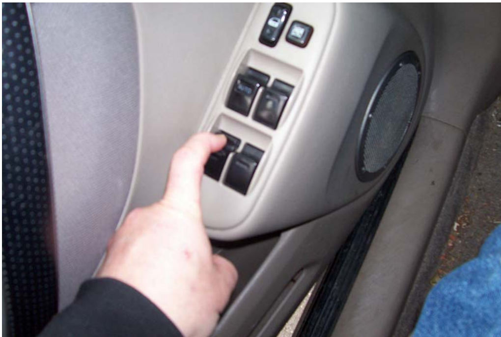
Exhibit 6. This photo shows an automotive pull-up/push-down power window switch.
