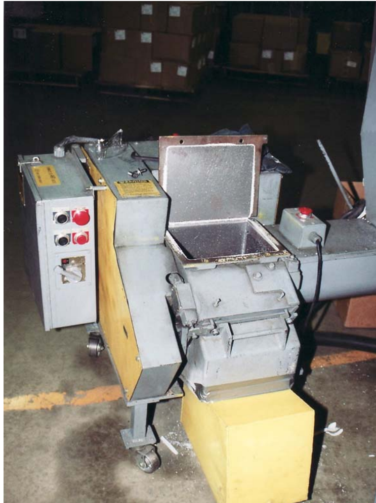
Exhibit 1. This photo shows an example of a machine interlock. The access panel is electrically interlocked so that the machine cannot be started when the panel is opened.
