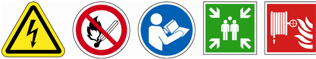
Exhibit 6. ISO safety sign vocabulary, left to right: warning sign, prohibition sign, mandatory action sign, safe condition/safety equipment location sign, fire safety sign
