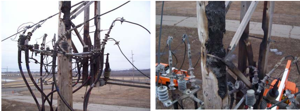
Figure 10. Tracking and Arching cause Pole Fire
