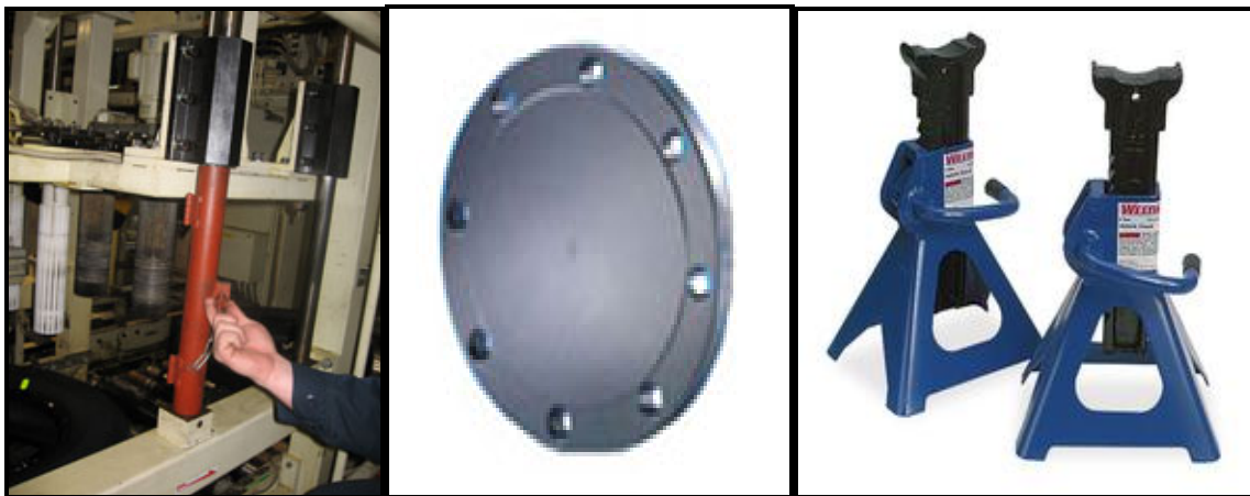
Figure 8. From left: Blocking an Equipment Press (photo 1); Pipe Blinding Flange (photo 2); Support Stands used for Blocks (photo 3)
