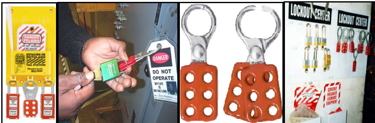
Figure 5. Typical Locks and Hasps for use in Locking Out Equipment
