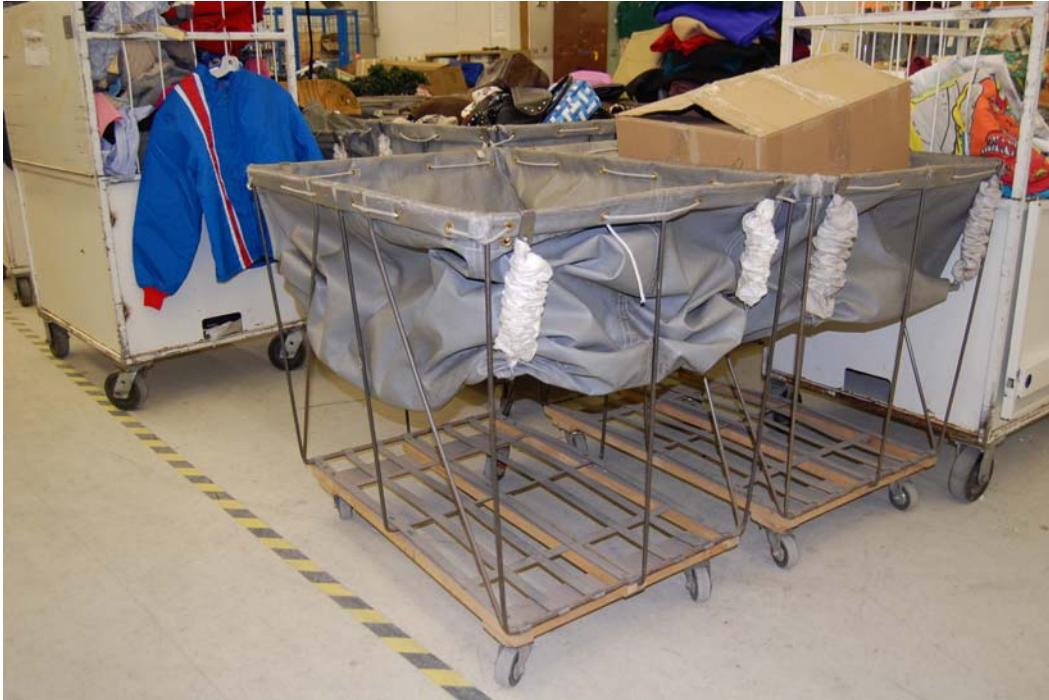
Figure 3. Spring-loaded totes are used so that the merchandise to be removed is always at waist height.
