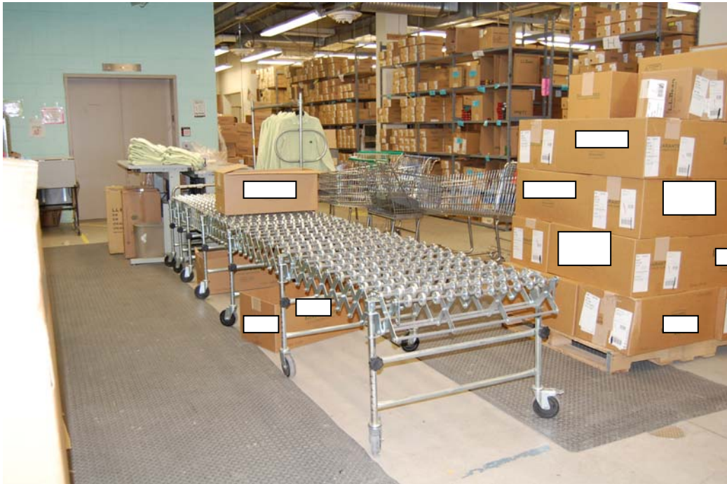
Figure 2. This photo shows an expandable skate wheel conveyor for unloading cartons. The height of the conveyors can be adjusted.
