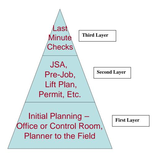
Figure 1. The Layered Approach to Hazard Recognition
