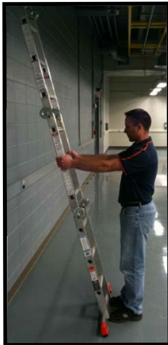
Figure 5. Positioning of Ladder at Proper Distance for 4-1 Ratio
