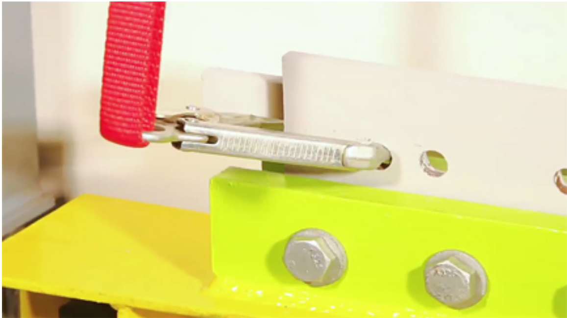
Exhibit 2. An example of transverse loading is pictured above.
