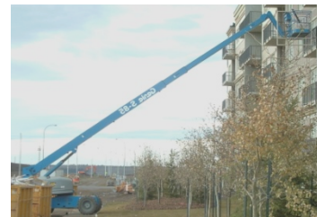
Figure 8 Boom Lifts may have a significant bounce when arresting a Fall
