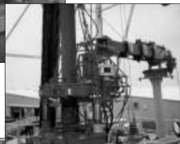
Mechanized equipment on the drilling rig has the following component groups: mechanized power tongs for casing, tubing and drill pipe (Photo 1, top); tong positioning systems for these mechanized tongs (Photos 2 and 3); and the stabberless system (Photo 4, left).
