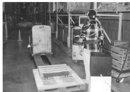
Photo 1: The LiftTrainer™ system used a magnetic motion measurement system. Cases were moved between the two scales sitting on the pallets.
