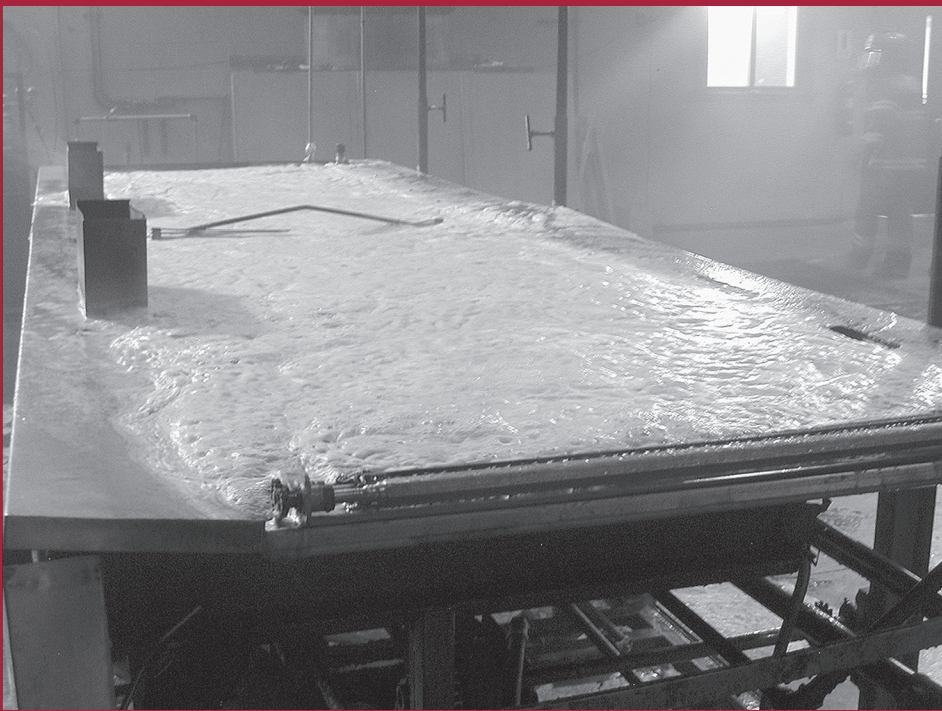
Photo 3 (left): Saponified kitchen appliance. Dry chemicals and the more recent wet chemicals extinguish oil and grease fires by forming a foam on the top. This foaming is a hydrolysis process in the fats called saponification.
