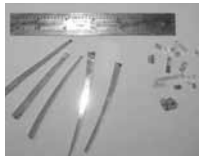
Photo 1 (left): Temper variations in a single sheet of automotive side glass shown by an impact test.
