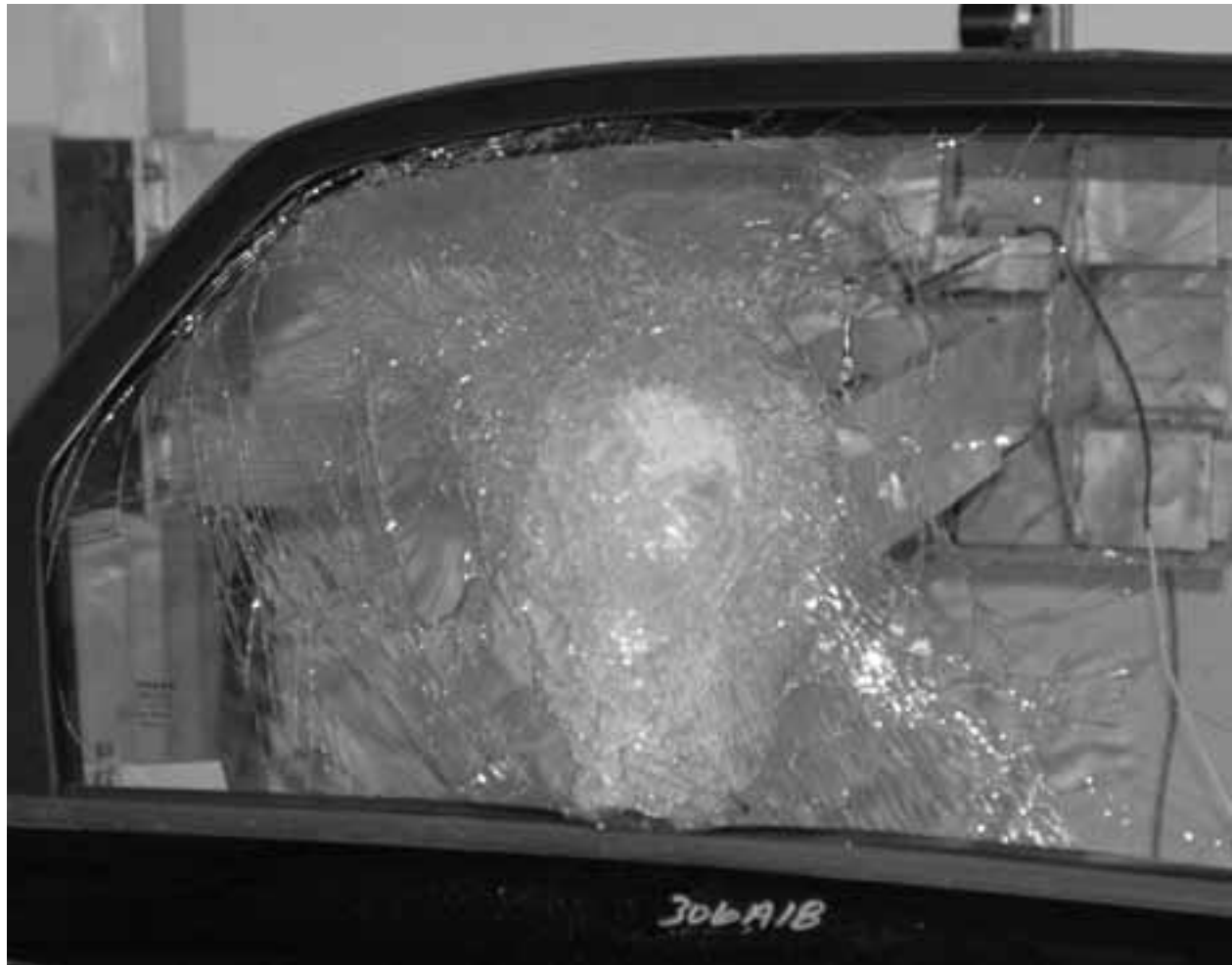
Photo 1 (left): Temper variations in a single sheet of automotive side glass shown by an impact test.
