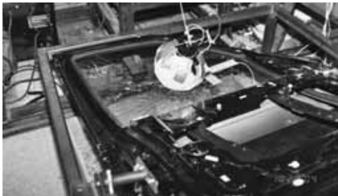
Photo 4 (below): Blunt headform impactor testing of commercial laminated side glazing.
