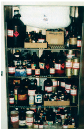
Photo 9 (above): A standard refrigerator being used for storage of toxic and flammable chemicals.
