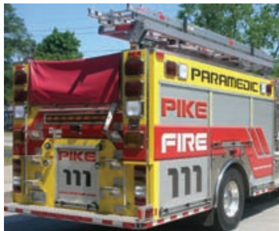
A typical fire truck carries the crew, pump, water tank, supply hose, ground ladders, handlines and other specialized equipment.
