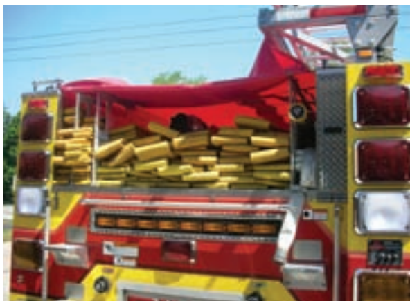
Hose carried on an engine includes large-diameter supply lines for connecting to hydrants and smaller-diameter supply line for "yard lays" to extend the reach of the handlines or supply portable master stream appliances.
