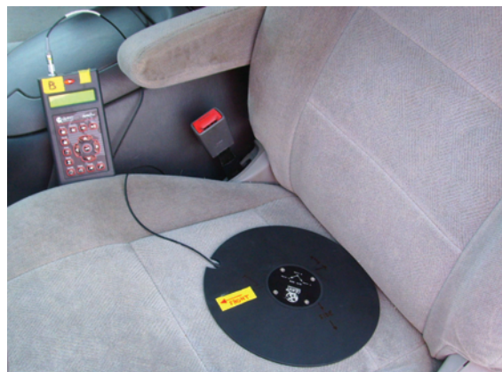
Photo 1: WBV monitoring instrument with a seat-pad accelerometer. Note the use of tape to mark direction and assist in the proper alignment of the seat pad accelerometer.
