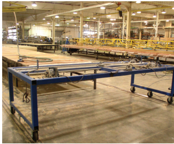
A saw cart (Photos 3 and 4) was recommended because it would automatically make the panel cuts—rather than having an employee make the cuts with a saw. This would isolate employees from the identified musculoskeletal risk factors.
