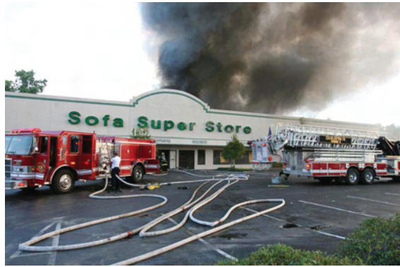
Photo 4: Water supply lines were extended from the nearest fire hydrants and hose lines extended far into the building. The kinked single supply hose in the foreground indicates inadequate incoming water pressure—resulting in inadequate water flow to the pumping engine.
