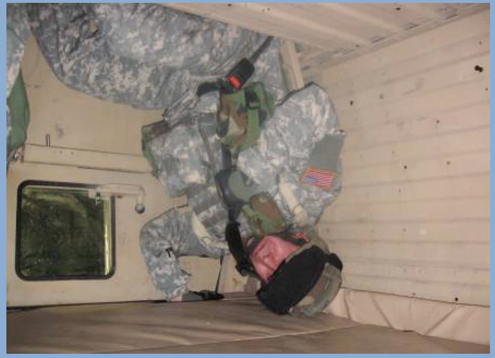
Photo 12: A soldier suspended by his seatbelt prepares to unbuckle as the HEAT rotation is stopped at the 180° point. Most soldiers have great difficulty during their first rollover in the HEAT.
