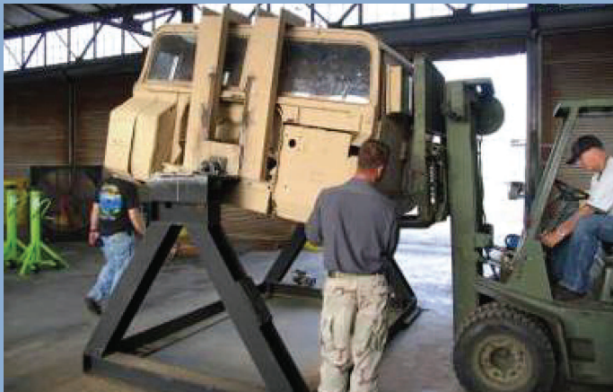
Photo 5: Jett, Hill and Whiting mounting the Humvee cab on the steel frame in an ECS 43 maintenance bay.
