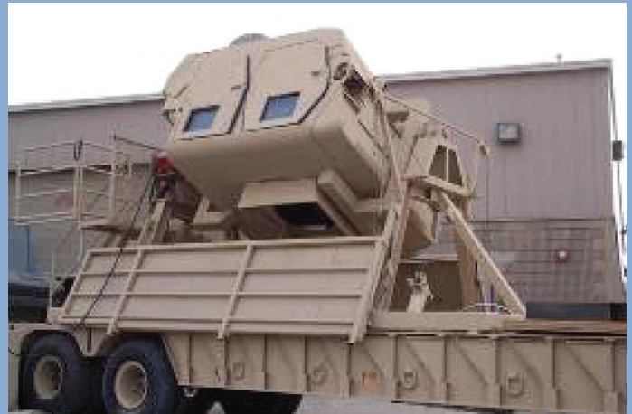
Photo 8: The trailer-mounted CFLCC version of the HEAT is fielded in Kuwait. Note the flip-down access platforms and safety guards.
