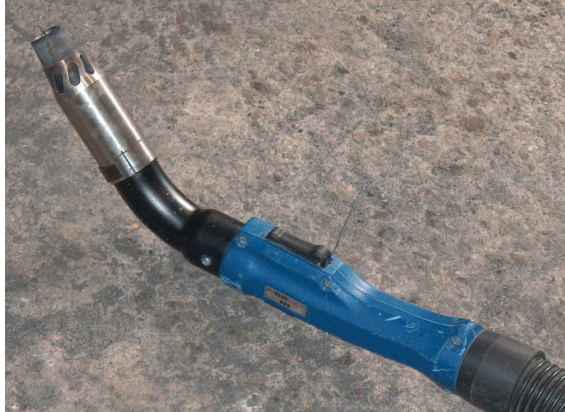
Photo 8: A fume extraction gun is one solution to the problems associated with frequently repositioning exhaust hoses.
