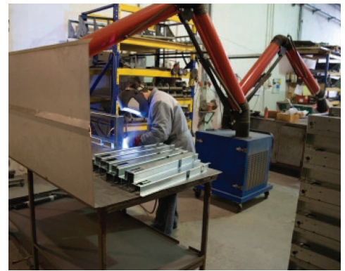
Photo 7: Portable fume extraction unit with movable extraction arms. Such a system provides more flexibility than backdraft welding booths.
