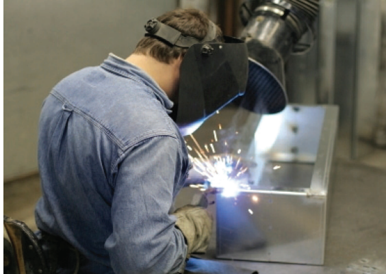
Photo 6: Local exhaust ventilation capture hood. These hoods come in various configurations and directly affect the capture efficiency.
