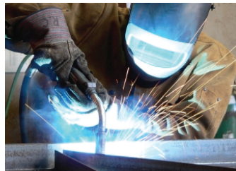
Photo 2: Gas metal arc welding.
