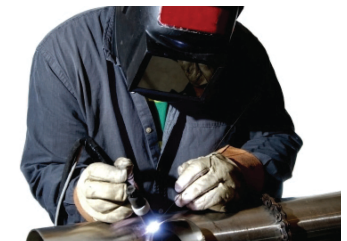
Photo 4: Gas tungsten arc welding.
