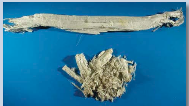
Photo 2: Asbestiform antigorite from Granada, Spain (upper), and Rowland Flat, South Australia (lower).
