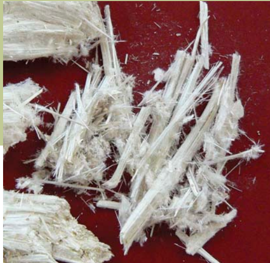
Photo 4: Asbestiform antigorite identified in a closed quarry near Rowland Flat, South Australia. From the 1940s to 1978, the asbestos was identified first as an amphibole variety of asbestos and later as chrysotile asbestos. This past decade, John Keeling, mineral systems team leader of the Geological Survey of South Australia, identified the strong presence of asbestiform antigorite in the quarry.
