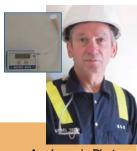
As shown in Photos 1 and 2, the datalogging instrument was taped into the upper pocket of coveralls and the remote sampling probe was positioned on the top of the shoulder. In this location, the device is protected and the alarm is easily heard.
