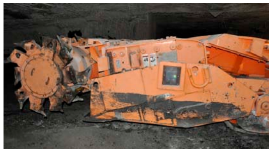
Photo 1: Example of a CMM showing the cutting drum.
