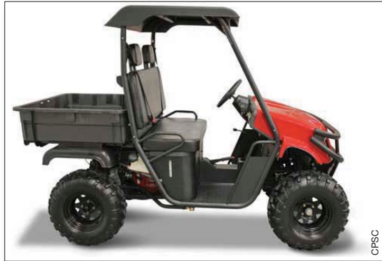
Photo 2 (top): A light utility vehicle fitted with a ROPS but with no passenger handhold on the upright. Photo 3 (bottom): "Wheelie bar" used on a tractor to stop a rear overturn.
