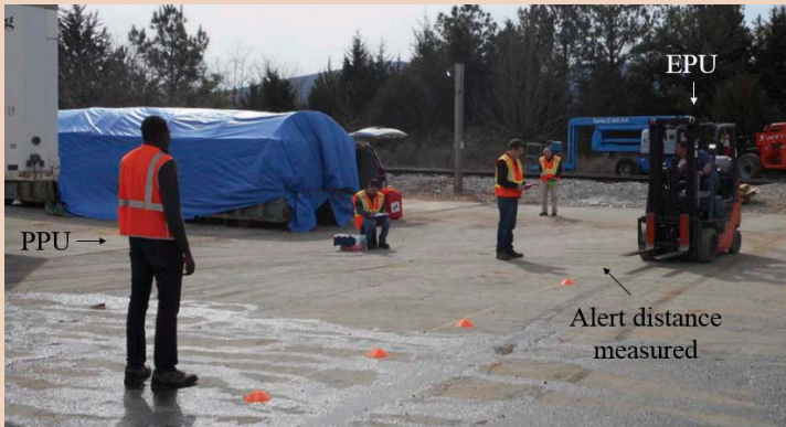
FIGURE 3 Test Bed for Mobile Forklift & Static Pedestrian Worker
