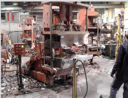
(Clockwise from top left) Photo 4: Aluminum die casting. Identified hazards include pinch points from die closing; tripping on debris on floor; impacts from turntable motion; and heat from molten aluminum and dies.
