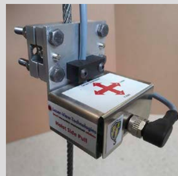
(From top) Photo 1: Boom angle indicator. Photo 2: Cable-mounted load moment indicator measurement unit. Photo 3: Load moment indicator display panel with alarms and lift-stopping mechanisms.
