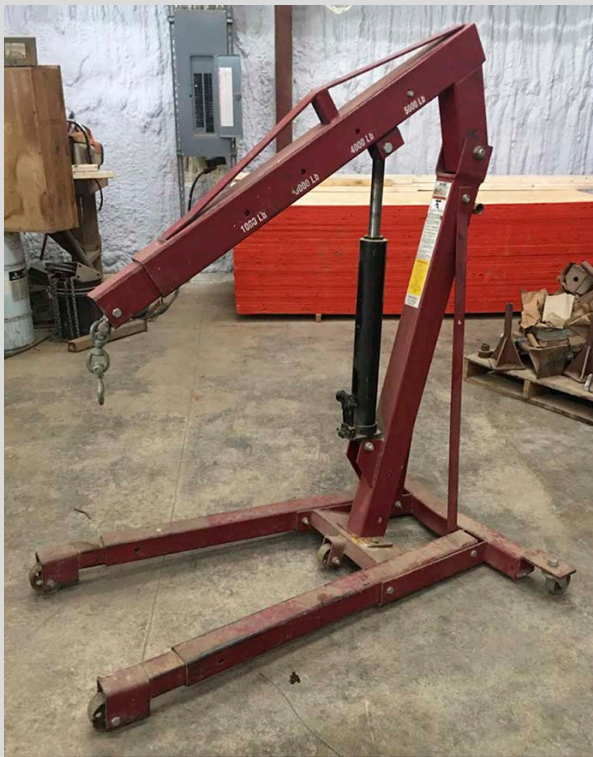
(From top) Photo 4: A 10,000-lb capacity portable gantry crane with hoist. Photo 5: 5,000-lb engine hoist.
