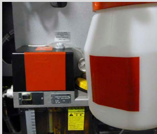
Photos 5, 6 and 7 are from the match game. Photo 5 (left) shows matching colors and shapes from the source to the portable container. Photo 6 (center) shows matching colors and shapes from the portable container to the machine. Photo 7 (right) shows mismatching oils.
