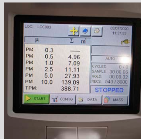
Photo 5 (below): Optical particulate measurement system results: 11.11 \mu\text{g}/\text{m}^3 size 2.5 \mu\text{m} ; 27.93 \mu\text{g}/\text{m}^3 size 5 \mu\text{m} ; 139.09 \mu\text{g}/\text{m}^3 size 10 \mu\text{m} ; and 388.71 particles per \text{m}^3 (0.388 \text{mg}/\text{m}^3 ) total particulate matter.
