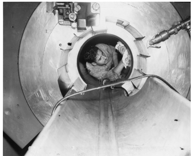
Photo 1: Man inside the barrel of a 16-in. gun. The photo was found in an album aboard the Battleship North Carolina .
